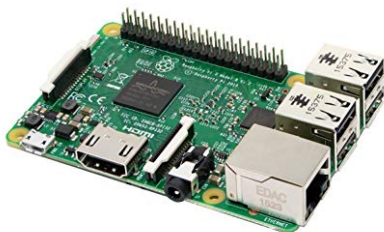
Figura: Broadcom BCM2837, encontrado no Raspberry Pi 3
